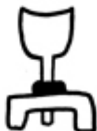
Figure 78 -- Possible way of mounting the small bell with a long handle and a bulb.
