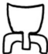
Figure 75 -- Unsuitable way of fitting the handle of a small bell directly into the stand.
